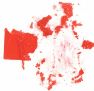
These are labels that literally destruct when removed. The label material breaks into tiny pieces when removal is attempted.
