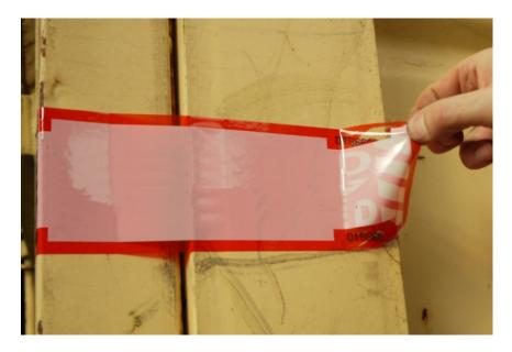
Container seals help maintain container integrity by protecting against insertion of unauthorised material and/or people and the removal of the cargo from pilferage and theft.
